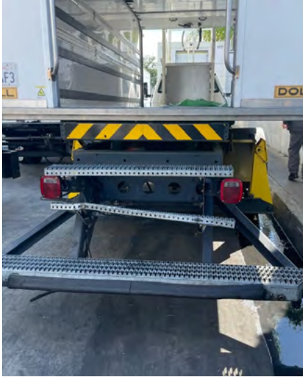
Broken loading steps on truck
